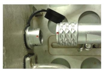
If connectors are connected properly the Recorder needs to be switched ON by placing the magnet (provided) at the designated position (marked on enclosure as ACTIVATE  $\,$ ). The left LED will be green and the right LED will be off indicating Recorder is in idle mode. Recorder has a self power down after  $\pm 2$  minutes if no communication was detected.
